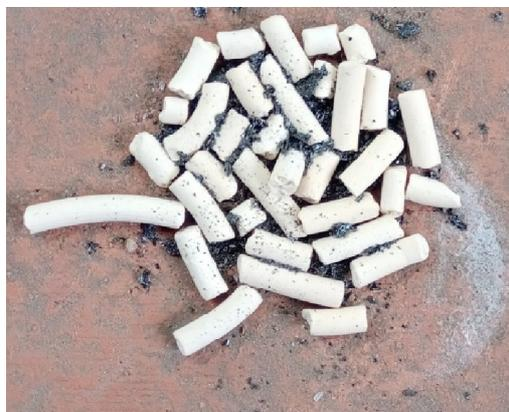
Figure 5. Char deposited HZSM-5 Pellets, 1:0.01, plastic to bentonite ratio
