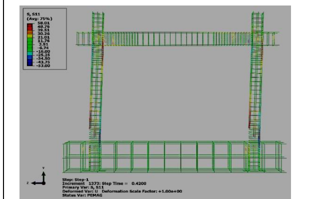
Fig. 6 Axial stress and tensile damage in DBF – 1
