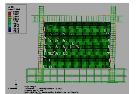
Fig. 7 Axial stress and tensile damage in NDFSM – 1
