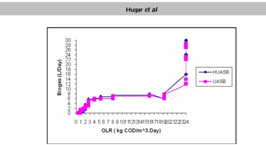
Fig 5: Observed biogas production for the fed OLR
