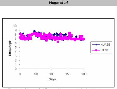
Fig 7: Variation of effluent pH observed during the study
