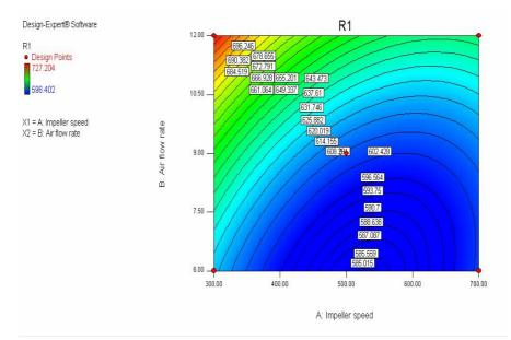
Fig 1 - Isoresponse contour plots showing the effect of impeller speed and air flow rate and their interactive effect on the volumetric mass transfer coefficient for 2 L sodium sulphite oxidation method.
